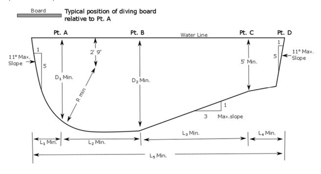
Note: L<sub>4</sub> is a minimum dimension to allow sufficient length opposite the board. This may of course be lengthened to form the shallow portion of the pool.
